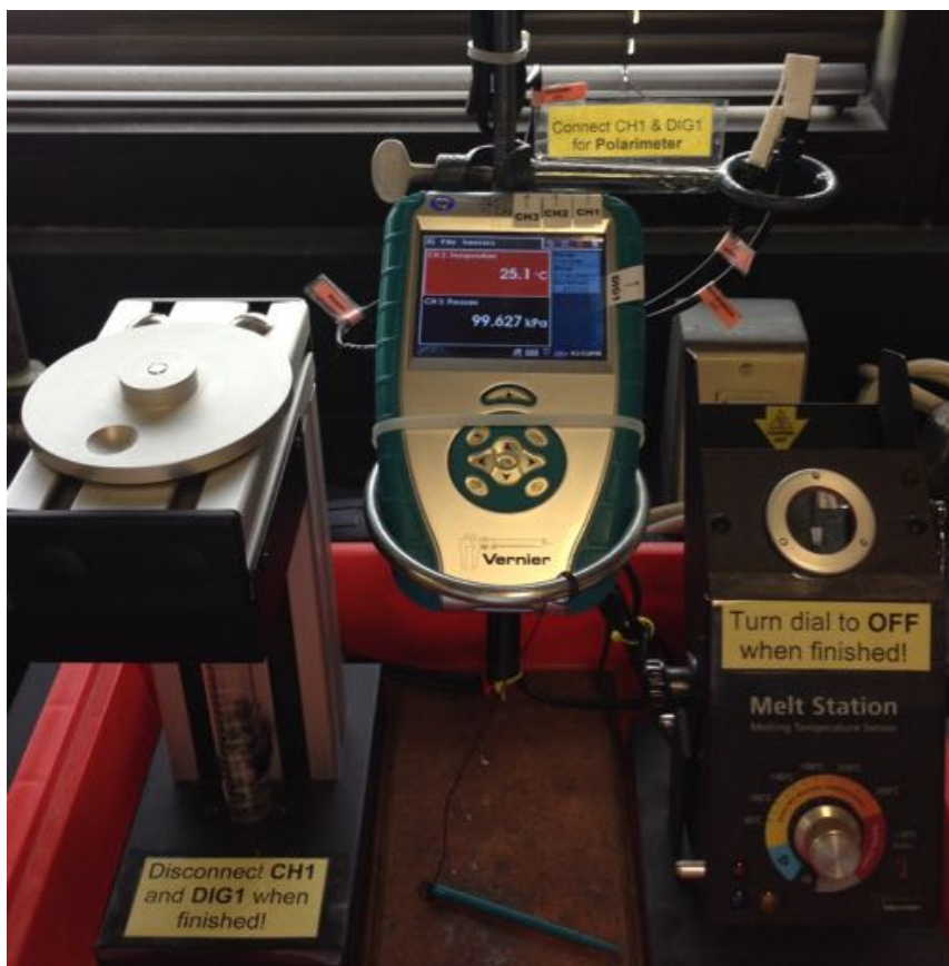
Figure A3.1: Vernier Polarimeter (left) connected to LabQuest interface (middle)
