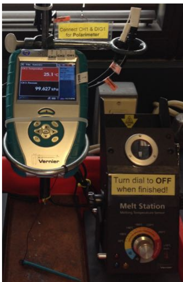
Figure A1.5: LabQuest Interface (left) and Melt Station (right).
