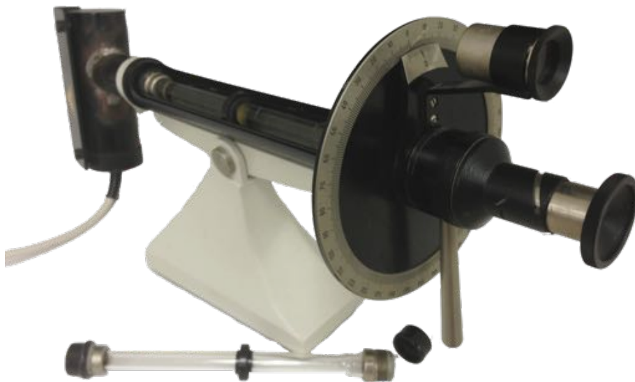
Figure A4.1: Laurent half-shade polarimeter with a vernier scale.
