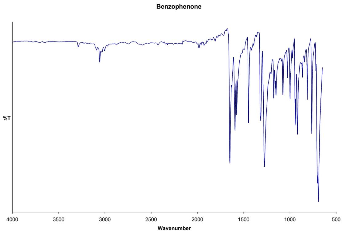
**Figure 31.1.** Infrared spectrum of benzophenone (neat)
