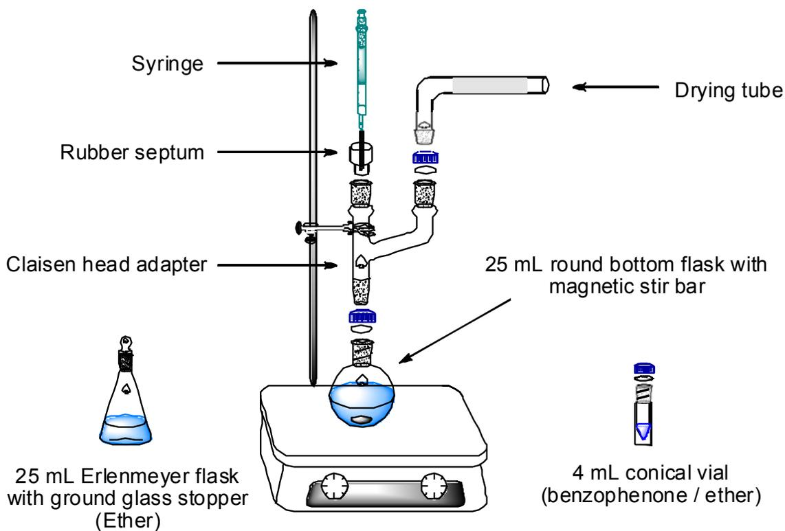
Figure 31.2. Apparatus assembly for the Grignard reaction.
