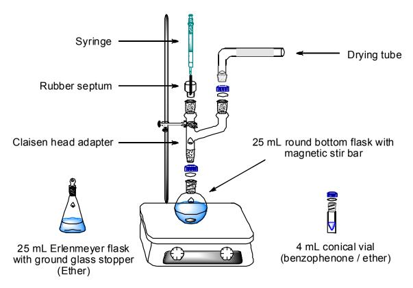
Figure 31.2. Apparatus assembly for the Grignard reaction.
