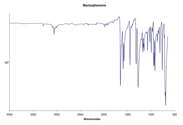
Figure 31.1. Infrared spectrum of benzophenone (neat)
